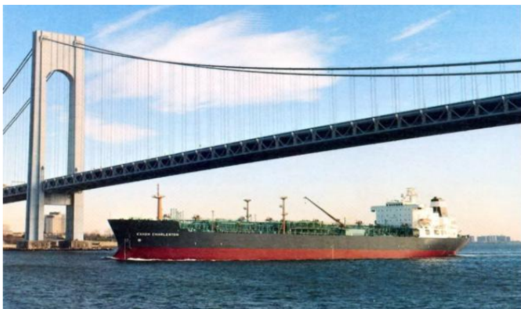
Exxon Charleston. LOA: 636 ft, Beam 106 ft, Draft 42 ft. Speed: 16.8 kts. Displacement: 62,500 tons. New owner 2004
